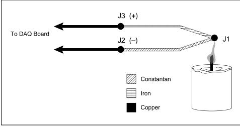
Figure 2. J-Type Thermocouple
